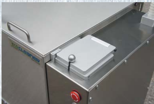
Filler port for adding new adsorber
