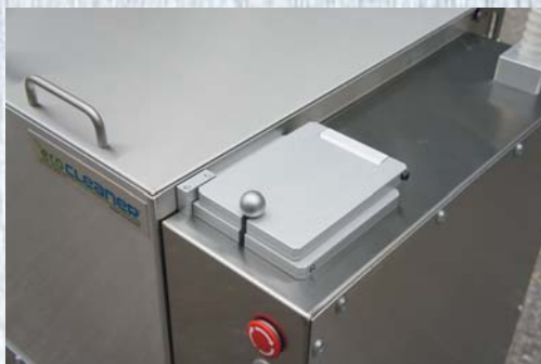
Filler port for adding new adsorber
