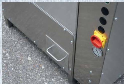
Easy access drawer to remove the spend adsorber
